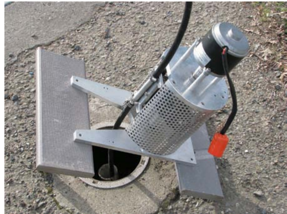
Pump rotated down onto well for pumping.
