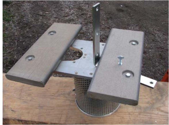
Front pontoon attached for above-grade mounting. Note set screw holding brace fully retracted.
