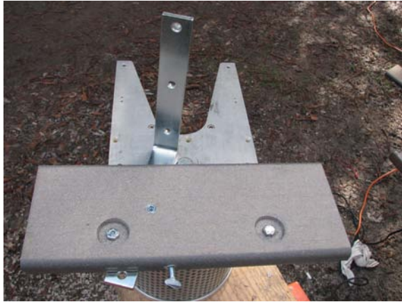
Rear pontoon and brace attached for above-grade mounting. Note storage location of set screw.
