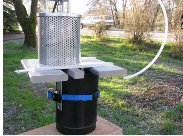
Pump mounted on 8 inch well surround (stove pipe). Pump rests on shim and front pontoon.
