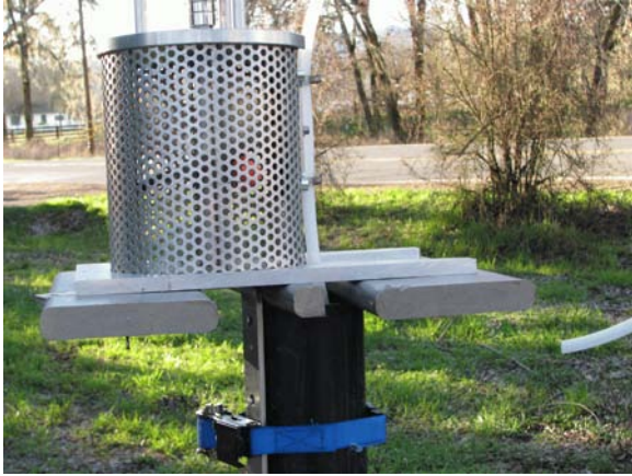
Pump slide backward on brace to position follower over pumping tube. Pump rests on shim and front pontoon on 4" well surround..
