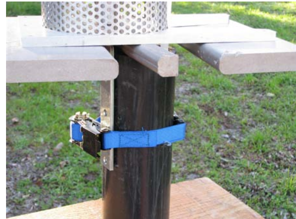
Pump brace strapped to well surround with ratchet and tape.
