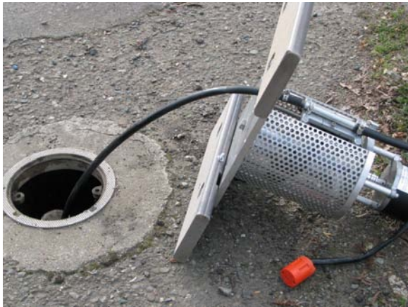
Pump rotated backward to permit easy attachment of pumping tube to follower.
